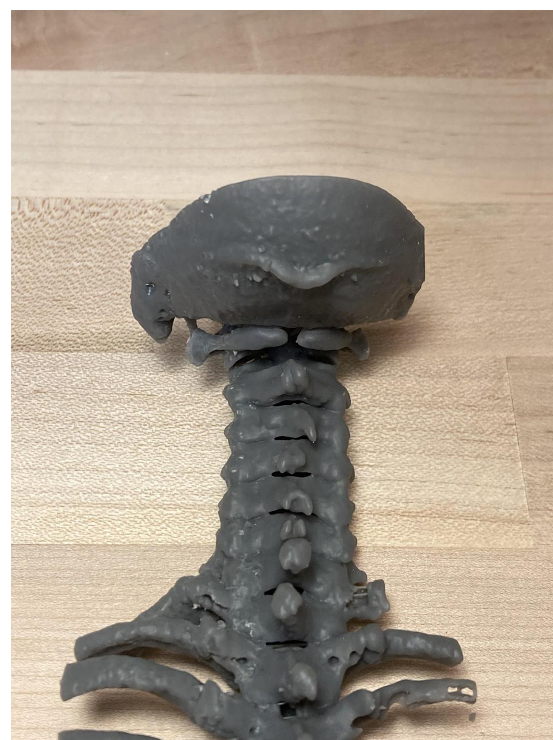
Figure 6: Presented below is the 3D print of the spine and occiput.
