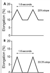
Figures A and B represent a cyclic short duration strain (CSDS) profile that previous researchers ( ) have developed to represent a repetitive motion strain.
